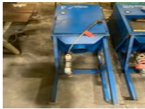
#568 • Donaldson Torit Mist Collector System Electric, 3ph, 208-460V.
