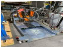
#553 • Parker Fluid Systems Hydraulic Oil Filter Cart
