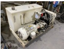
#589 • Hydraulic Power Unit Powered by an electric, 3ph, 230/460V industrial motor.
