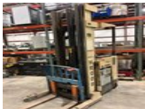
#434 • Crown 36V Narrow Aisle, Stand-Up Reach Forklift
